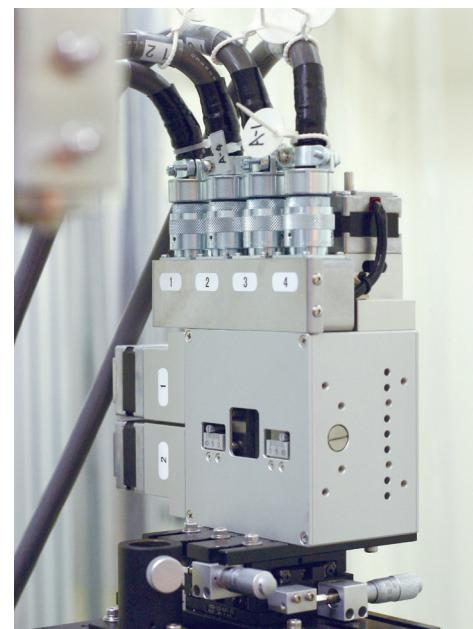
Easy use for each blades actuated by motors. More than 12 slits were installed in synchrotrons in recent 4 years. This is more precise than GHM-13B.
