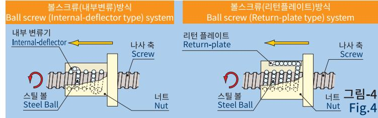
The ball screw consists of a screw spindle, a nut, and steel ball between them (Fig. 4). When the screw is rotated, the ball rolls and moves between the ball screw and the nut, and then returns to its original position. Since a ball is rolled, the friction is low, a high transmission efficiency is obtained, the difference between static friction and dynamic friction is small, and stick-slip does not easily occur.
