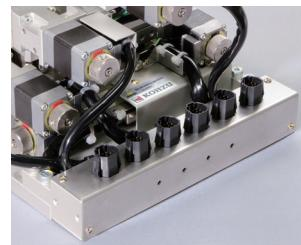
The 6-axis motor and sensor wiring are concentrated in one location to make even complicated multi-axis wiring work easy (can also be removed if not needed).
