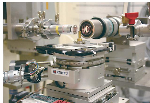
This Picture is shown as X-ray CT with SPU-1A for analysis of collected particle from Itokawa asteroid, Japanese Hayabusa mission (photo SPring-8).
