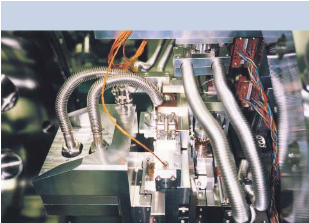
APM-2 monochromator : cooling tubes inside vacuum chamber.
