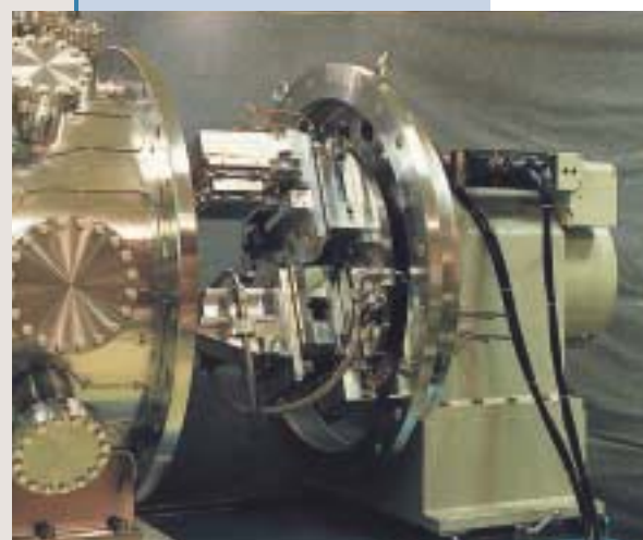
Crystal adjustment mechanics of HLD-1 monochromator.
